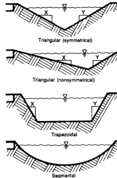
Figure 6-23. Ditch cross sections
