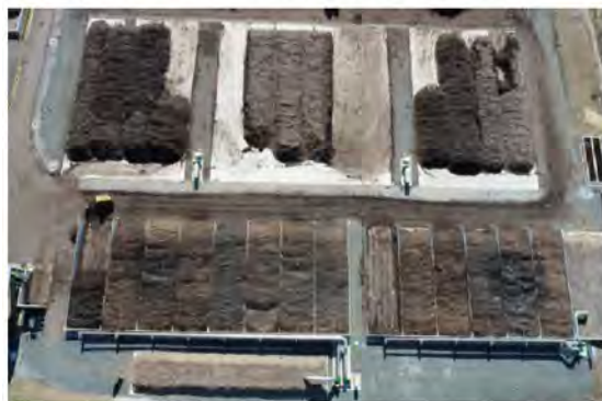
Figure 3-7 Example of Reversing Extended ASP Primary and Walled Secondary (80,000 tons per year capacity)
