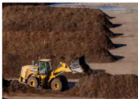
Figure 3-4 Example of Front-end Loader Managed Windrow
