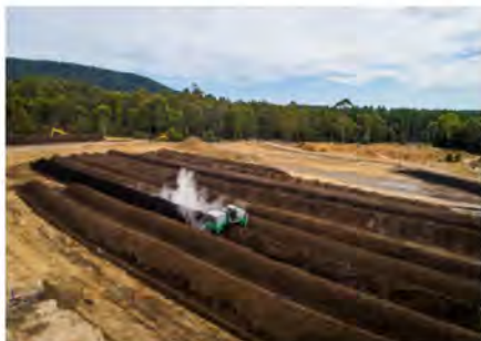
Figure 3-6 Example of a turned-windrow composting operation
