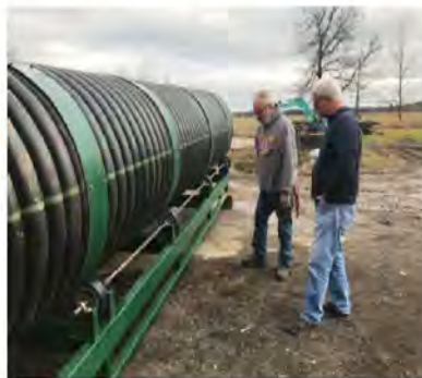
Figure 3-15 In-vessel Drum Composter in the Town of Newcomb
