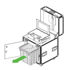
3. Use key to open the Ballot Box Door in the front of the machine and verify no ballots are in the ballot box. If you find any ballots remove them, place a big X on them, fold in half, and put in the Blue Inspector bag. Be sure to leave the ballot box open and return it to the inside of the machine, slide all the way to the left. Close and lock the door. Seal the door with a Red String Seal and record on the Seal Report.
